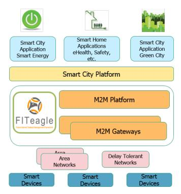
Figure 1. Smart City Reference Architecture.
