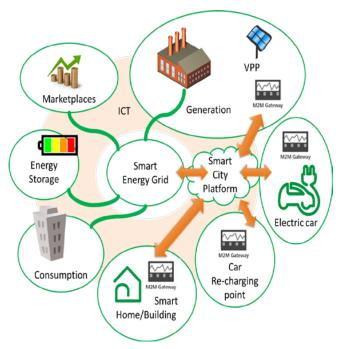
Figure 3. System model of the electricity grid using the Smart City platform to accommodate new services like searching for the nearest free electric car re-charge point
